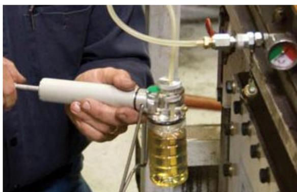
Current method of oil sample extraction from hydraulic equipment.
