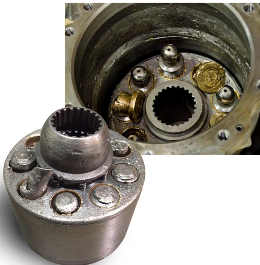
UPPER-RIGHT: Catastrophic hydraulic motor failure due to contamination.
