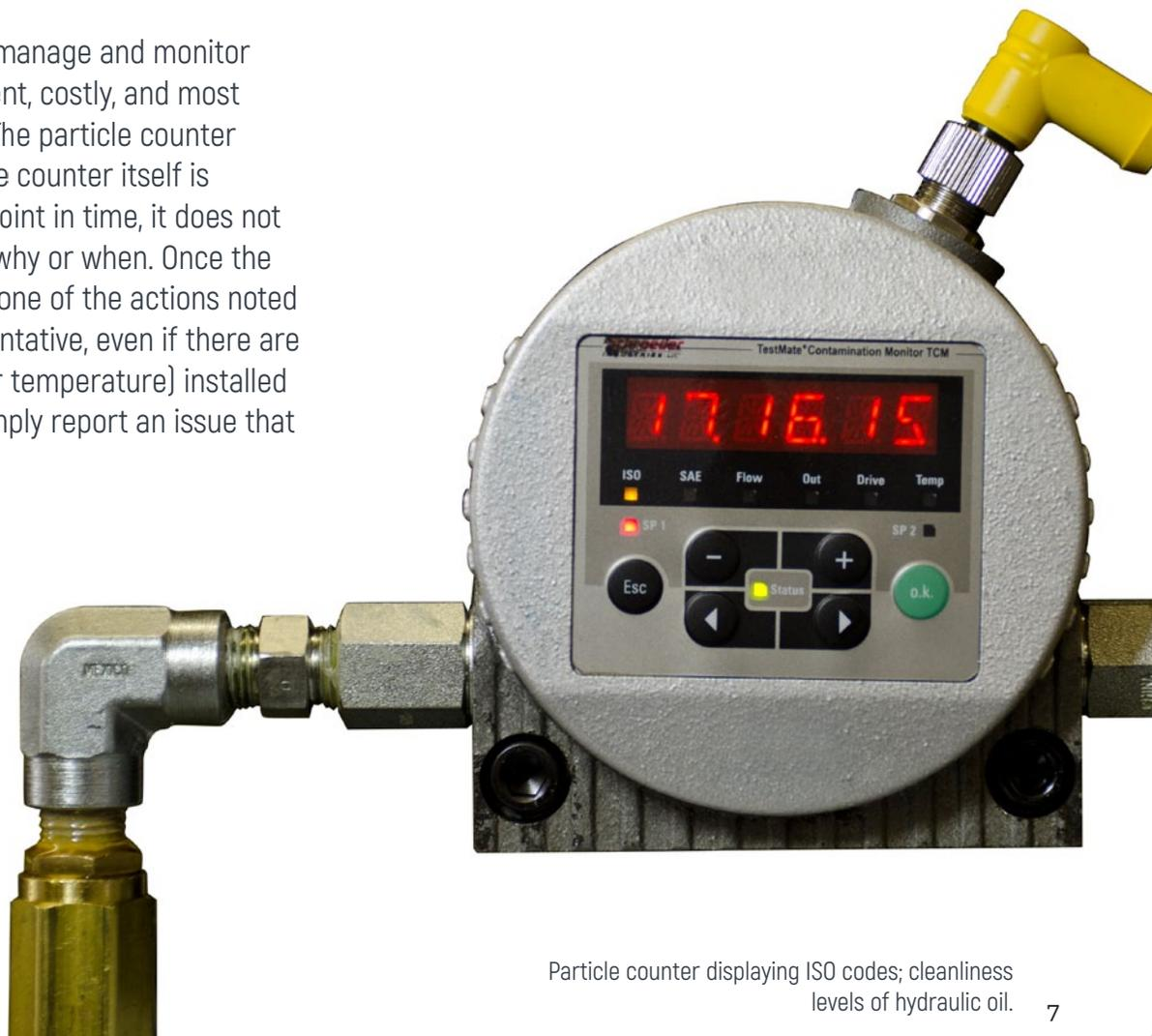
Particle counter displaying ISO codes; cleanliness levels of hydraulic oil.
